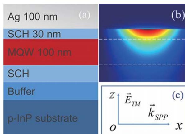
FIG. 1. (a) The schematic configuration of the Ag/InGaAsP Schottky SPP-emitting diode. MQW: multiple-QW. (b) The electric-field distribution of the fundamental surface plasmon mode. (c) The electric field direction for the TM modes and the propagation direction of SPPs.
